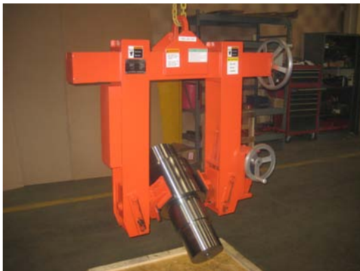
1,500-pound hand wheel operated rotating axis grab lifts and rotates machined gearbox parts around their horizontal axis.
