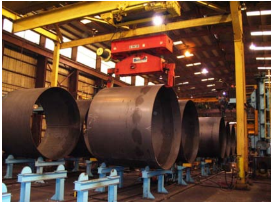
Grab for lifting and rotating pipe (tower) sections
