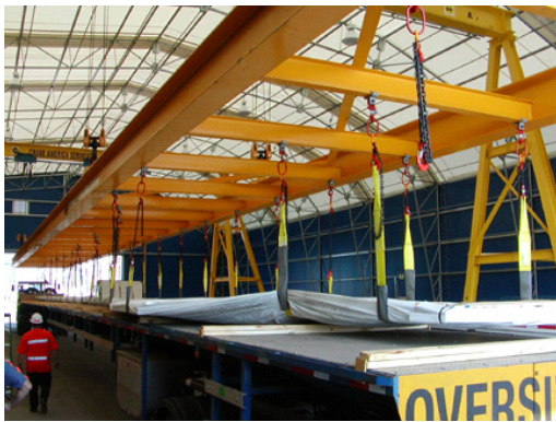
Extra long and extra wide spreader beams for handling towers and blades
