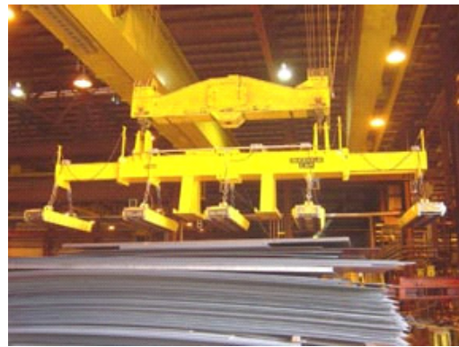
Telescoping plate handling magnet beams
