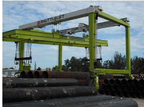
Hydraulically adjustable spreader beams for outdoor storage
